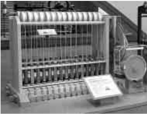
The model of the traditional, manually operated Garabo spinning machine, 1873.
